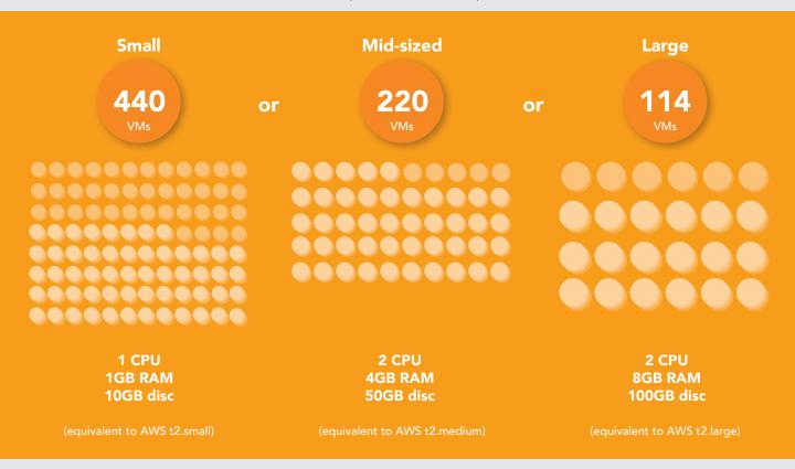
Illustration assumes 50% disk utilization, 50% CPU over-provisioning and 10% virtualization overhead.
